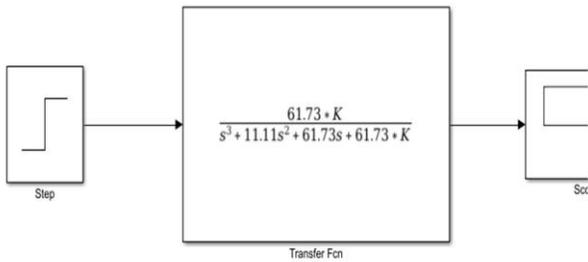
Figure 5: Reduced transfer function
