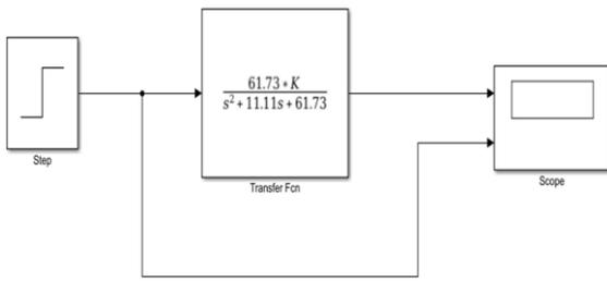
Figure 4: Open loop transfer function
