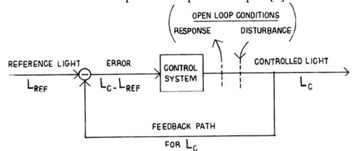
Figure 2: A schematic human eye as a servo-mechanism [2]
