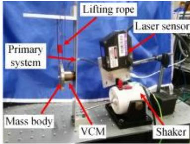
Fig. 4. The experimental setup (a) Schematic diagram of the experimental set-up (b) Photograph of the experimental set-up [10]
