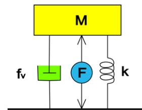
Fig. 7. Schematic diagram of floor vibration controller.
