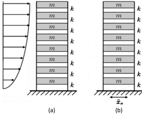
Fig. 2. a) wind excitation b) earthquake excitation [4]
