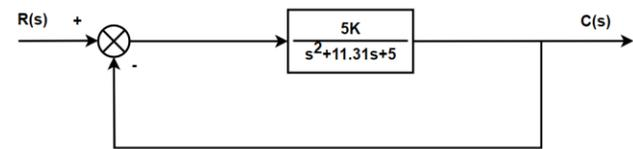
Fig 20. Equivalent transfer function block diagram.
