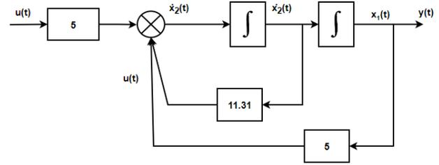
Fig. 9. Gain/ Signal attenuation diagram.
