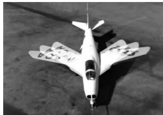
Fig 6 Variable Sweep Morphing in a Bell X-5 [17]
