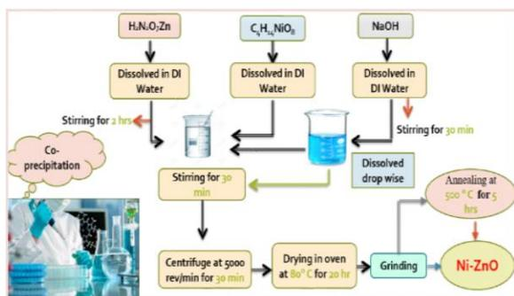
Fig. 1. Synthesis route for  $Zn_{1-x}Ni_xO$  NPs.
